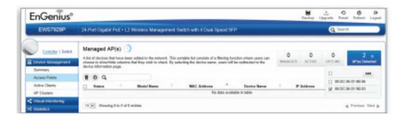
Step 2: To manage the Managed AP(s), select the desired Managed AP(s) by checking the boxes and click **Add**.
